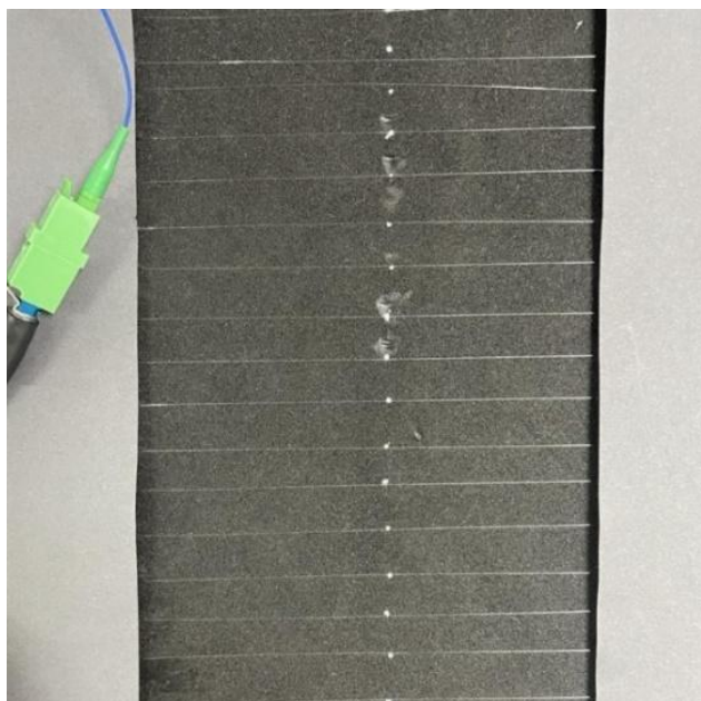
Figure 2. Temperature sensor setup. Fiber divided into 20 segments.
