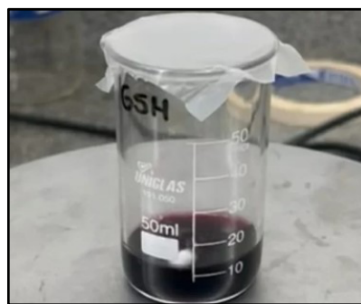
Figure 5: Reaction after synthesis with GSH/NaBH 4 .
