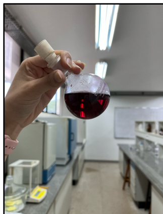
Figure 3: Reaction after synthesis with sodium citrate, containing gold nanoparticles formed.
