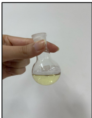
Figure 2: Aqueous solution of gold ions before the start of the nanoparticle synthesis reactions, showing the initial state of the material before reduction.
