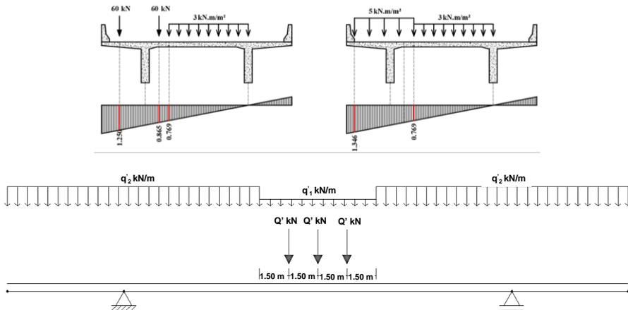
Fig. 1 2D procedure for the load effects estimative in bridges. Live loads and influence lines in the cross-section, and longitudinal loads.
