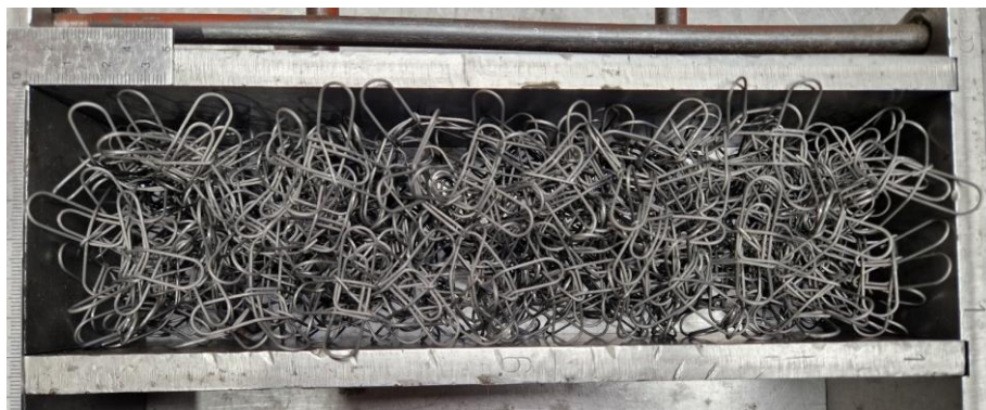
c) Complete filling of a formwork (70×70×250 mm) with the new reinforcing elements
