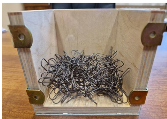
b) Partial filling of a cube mould of 100 mm side lengths with the new reinforcing elements
