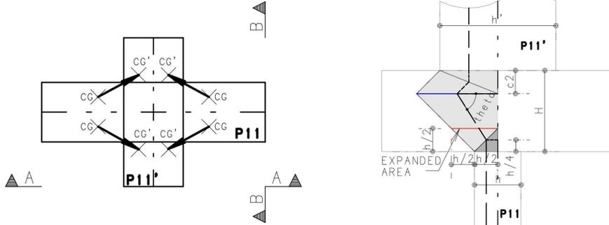
Fig. 3 Direction of the Load Path in Model 2 | Section BB: Model 2
