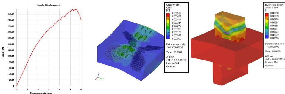
Fig. 8 Load x Displacement | Cracks and Deformations of the Nonlinear Model at Failure
