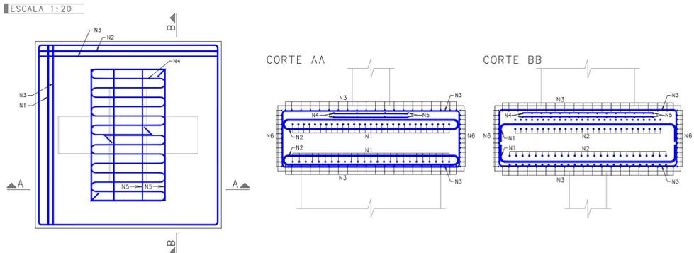
Fig. 6 Detailing of the Transition Block
