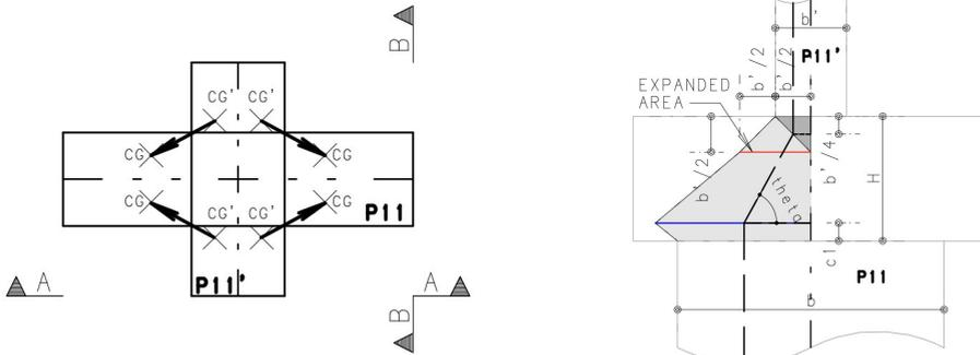
Fig. 2 Direction of the Load Path in Model 1 | Section AA: Model 1
