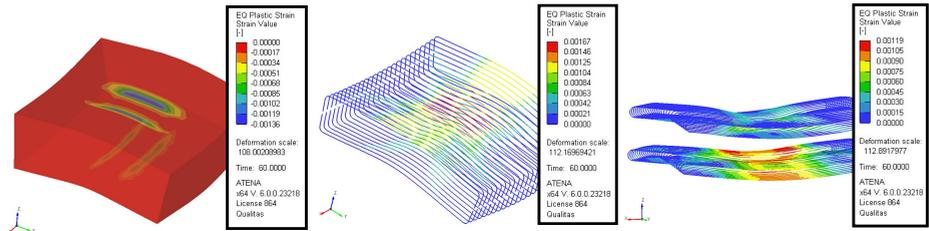
Fig. 9 Concrete and reinforcement deformations at failure
