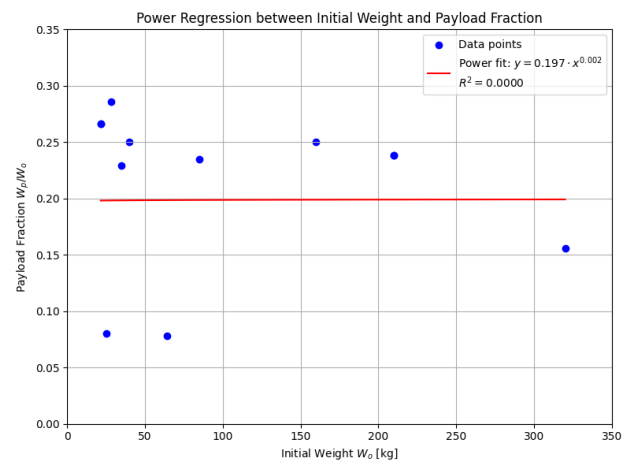
Figure 5. Payload weight percentage based on historical trends and benchmarking. W p : payload weight; W 0 : take-off weight; y: power-type trend line; R 2 : coefficient of determination.
