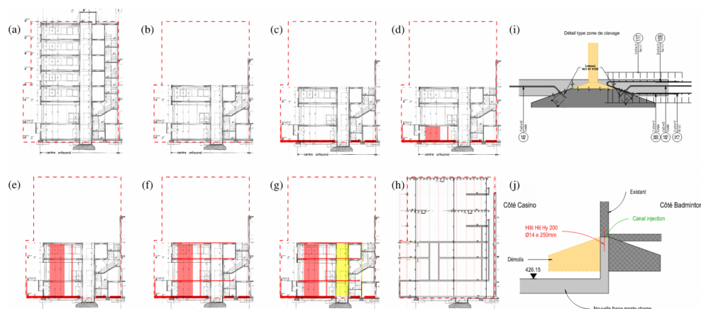
Fig. 12 Construction sequence: (a)–(g) sequence in ground floors; (h) construction of upper floors; (i) reconnection between foundation slabs after wall demolition; and (j) underpinning construction under Badminton middle-wall
