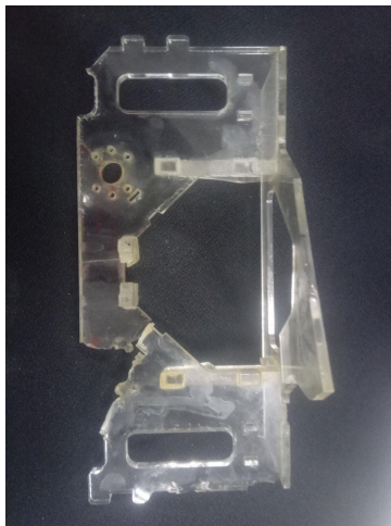
Figure 2. The acrylic structure supporting the thrusters was damaged.
