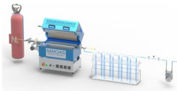
Figure 1 - Equipment used on the pyrolysis process.
