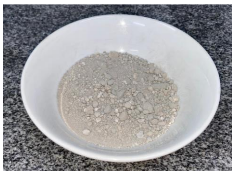
Figure 1. Photocatalytic titanium dioxide residue used in the mixtures.
