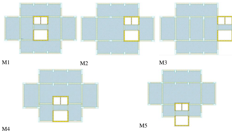
Fig. 3 Models studied by varying the position of the concrete core in the plant.
