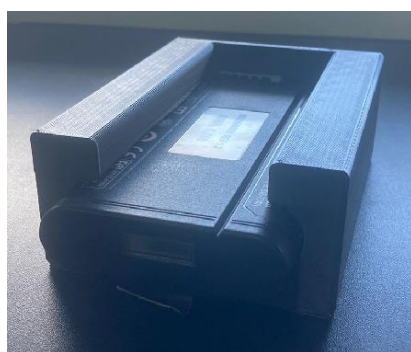
Figure 3. Battery installed in the printed mount.
