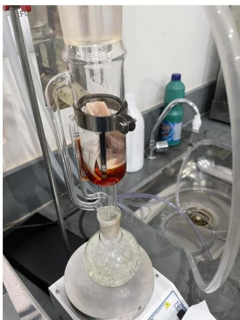
**Figura 1.** Extrator de Soxhlet
