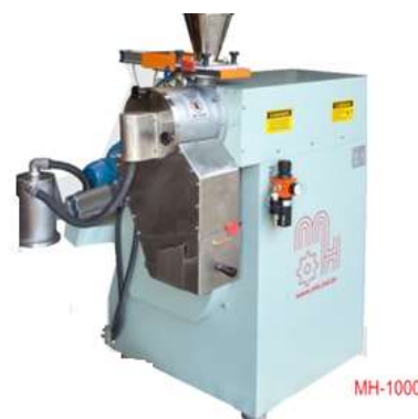
Figure 1. Thermokinetic Mixer (DRAISS Homogenizer)
