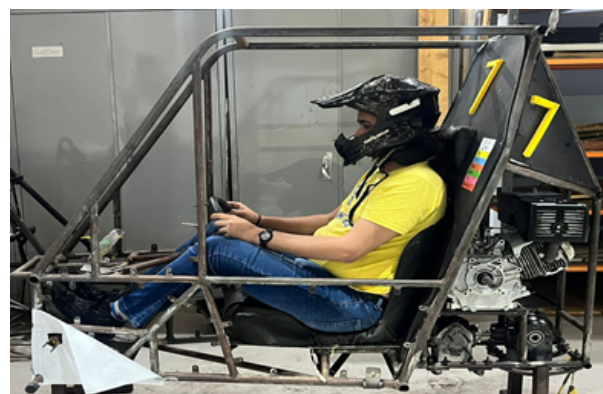
Figure 7: Photogrammetry of the ninety-ninth percentile male in cockpit prototype.
