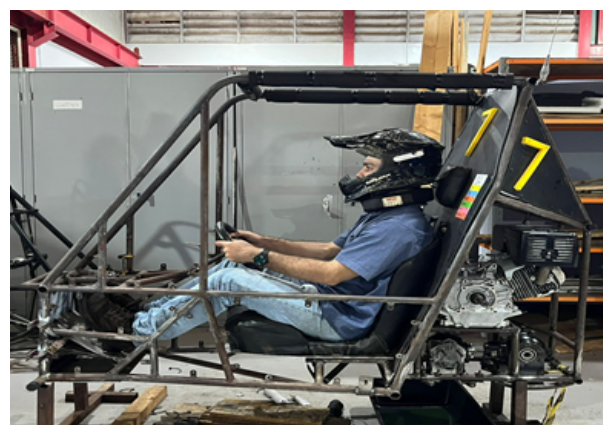
Figure 6: Photogrammetry of the forty-second percentile male in cockpit prototype.
