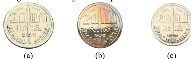
Figure 3. Images of silver 500 coins. In (a) control; in (b) coin without coating after exposure to \text{H}_2\text{S} atmosphere for 24 hours; and in (c) coin with coating after exposure to \text{H}_2\text{S} atmosphere for 24 hours.
