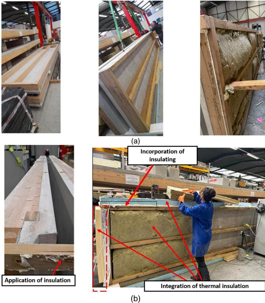
Fig. 2. Test conditions: (a) Setup of the tested panels; (b) Installation of the insulation.
