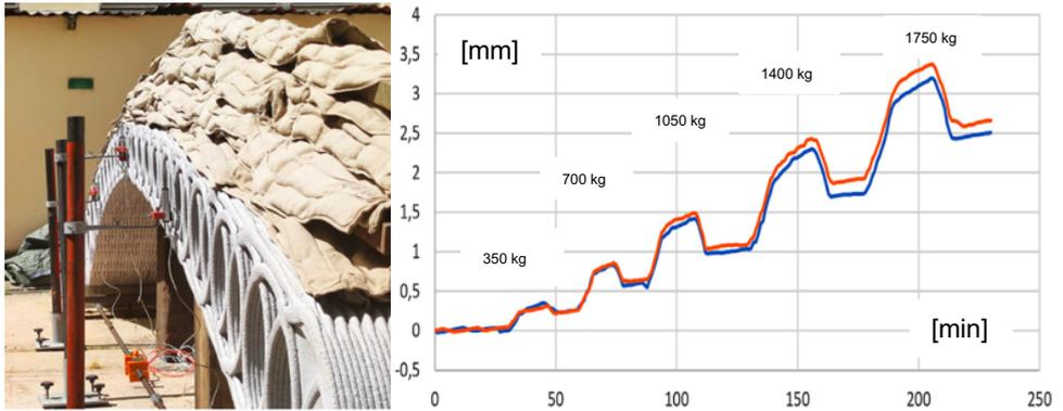
Fig. 5 Load bearing test of the footbridge. Loading diagram.
