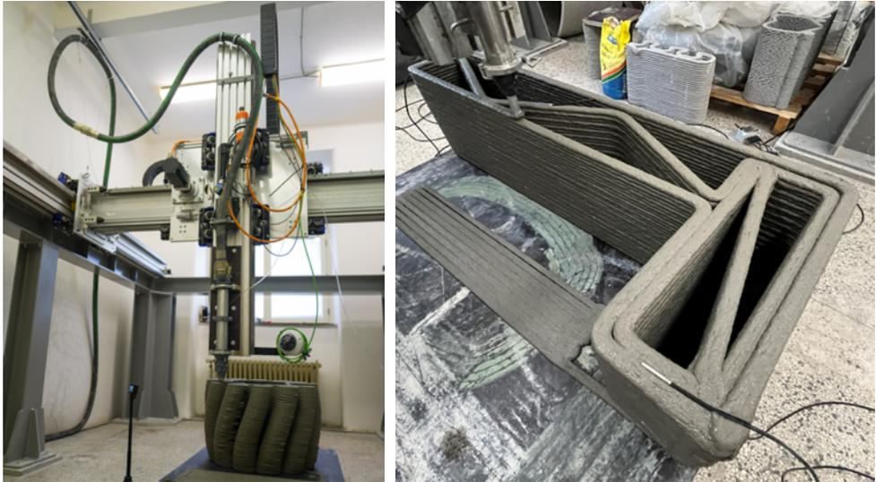
Fig. 1 TestBed – printing device (left), example of printing setup (right)
