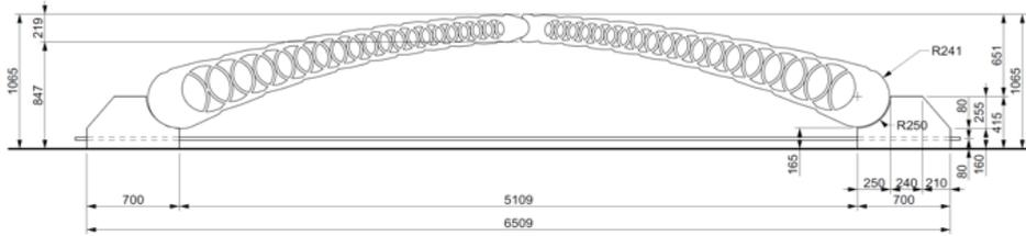
Fig. 4 Final footbridge design drawing
