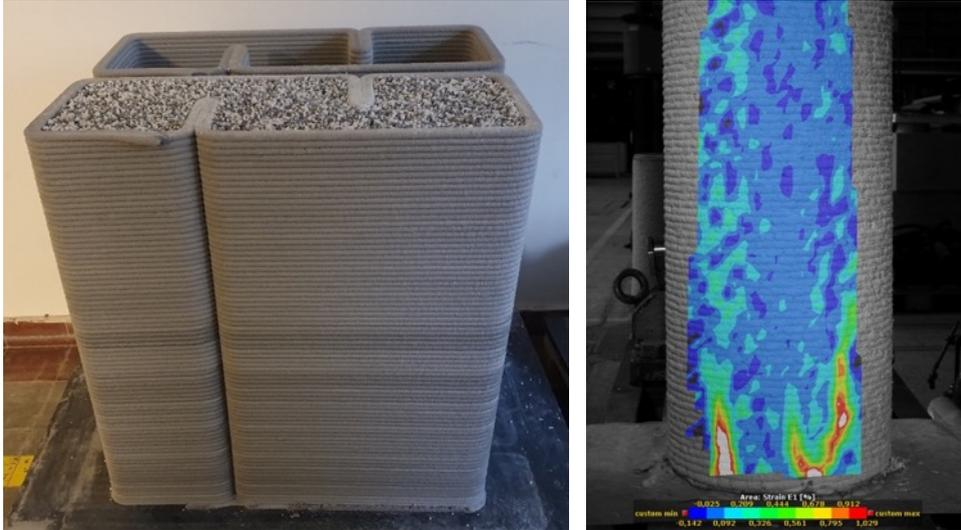
Fig. 2 Experimental wall specimen (left), image from DIC during 3D printed column
