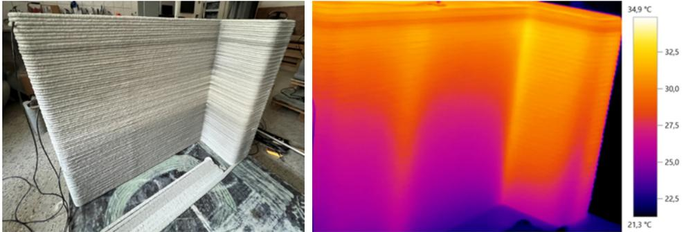
Fig. 3 Experimental wall specimen (left), image from thermocamera
