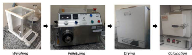
Fig. 1. Scheme of the conformation process. From left to right: 1- Analytical balance; 2- Pelletizer; 3- Stove; 4- Muffle. *Adapted from [4].
