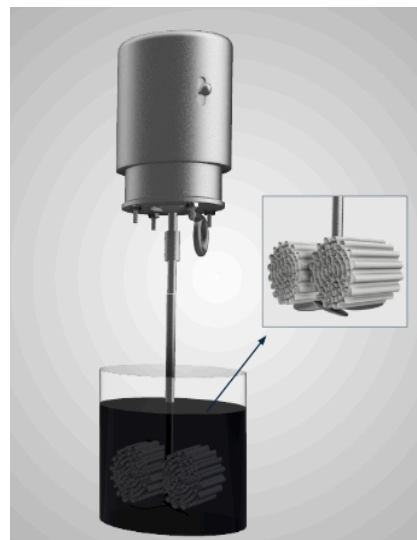
Fig. 1. Schematic illustrating the batch system used in the RB5 dye adsorption tests.
