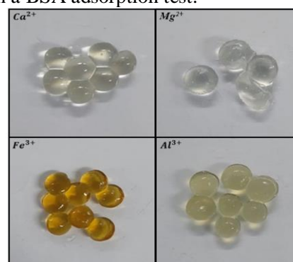
Fig. 3. Adsorbents after 60 minutes of agitation at 25°C in a BSA adsorption test.
